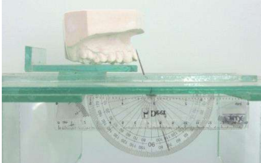
Figure 1: TIP with a dental cast mounted, ready for measurements to be taken.
